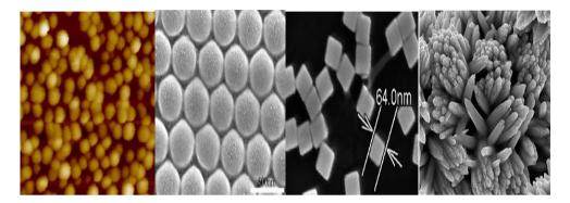
Fig.1. (i) Gold nanoparticle, (ii) FePtnanosphere, (iii) Silver nanocubes, (iv) Titanium nanoflower
